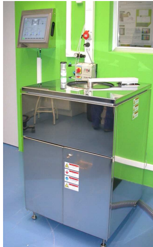
Figure 1. Atomic Layer Deposition equipment used to obtain nanocoatings
